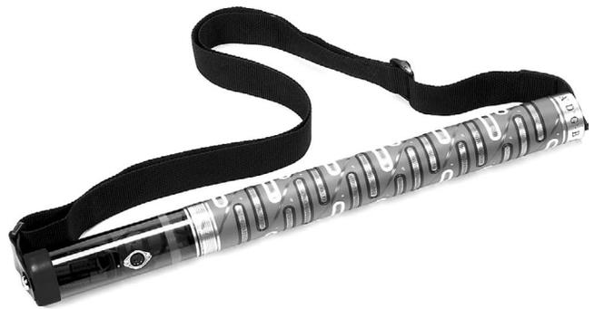
**Figure 4.22.** *The Continuum Fingerboard tracks and updates MIDI values for the x, y, and z positions of one to sixteen fingers every 1.33 milliseconds; these values appear at the MIDI Out as well as the FireWire® port. (Courtesy of Haken Audio, [www.hakenaudio.com](http://www.hakenaudio.com).)*
