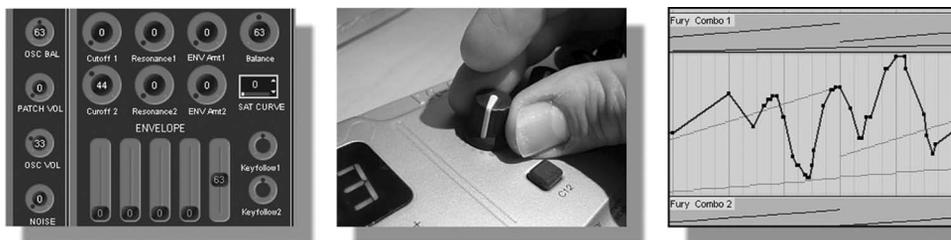
**Figure 5.21.** Examples of how a controller value can be varied as parameter faders, physical hands-on controls, or drawn parameter curves.
