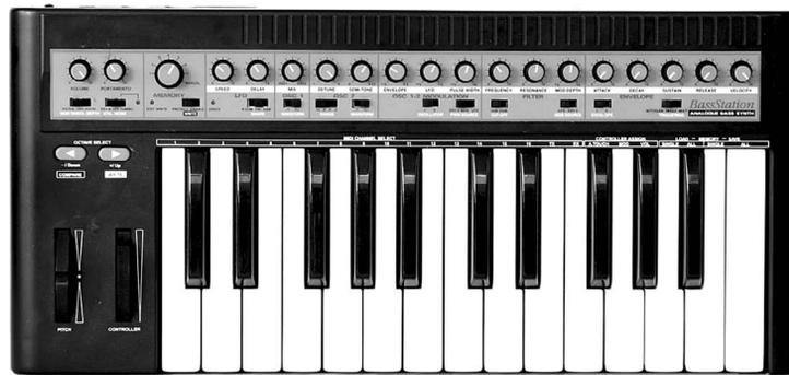
like the waveforms, vary over time. Subtractive synthesis makes extensive use of filtering to alter and subtract overtones from a generated waveform (or series of waveforms). For example, such a device could start with a square or sawtooth waveform that, with the use of filters, could be altered to approximate an acoustic instrument. These generated sounds can also be filtered and changed in level over time to more closely approximate a desired sound.
