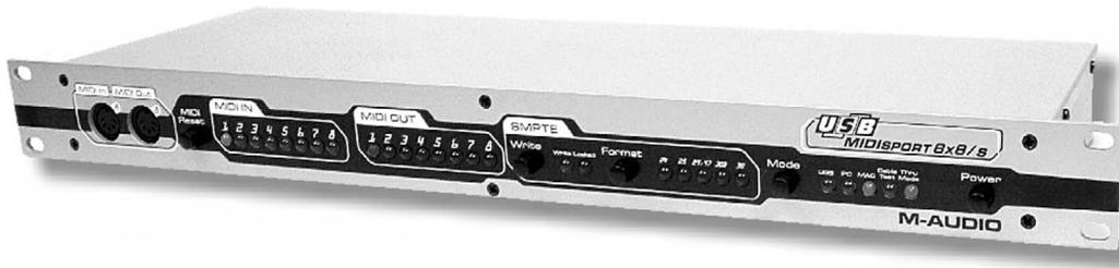
**Figure 3.17.** M-Audio MIDISPORT 8 × 8/s MIDI interface. (Courtesy of M-Audio, A Division of Avid Technology, Inc.; [www.m-audio.com](http://www.m-audio.com).)
