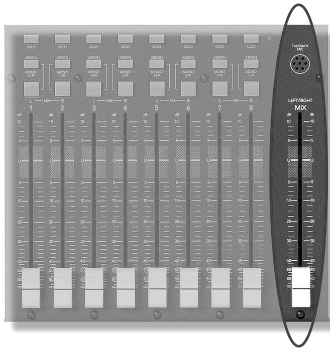
controls are horizontally duplicated across a console's surface. These gain controls are physically tied to an auxiliary send bus that routes the mixed levels to an output destination. The main stereo or surround buses feed to the channel faders and pan positioners and then onto the mixers main output buses, which are combined with the various effects return signals and routed to the monitor speakers and/or recording device.
