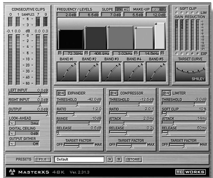
In addition to the basic complement of dynamic range processors, wide assortments of multiband dynamic plug-in processors (Figure 6.45) are available for general and mastering DSP applications. These processors allow the overall frequency range to be broken down into various frequency bands. For example, a plug-in such as this could be inserted into a DAW's main output path which allows the lows to be compressed while the mids are lightly limited and the highs are de-essed to reduce sibilance.
