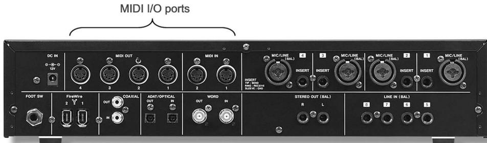
**Figure 3.15.** Most audio interface devices include MIDI I/O ports. (Courtesy of TASCAM, [www.tascam.com](http://www.tascam.com).)
