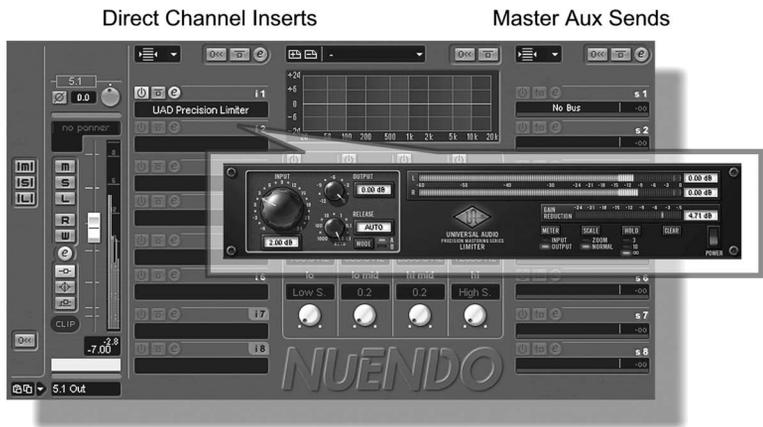
of multiple plug-ins become a drain on your CPU (something that can be monitored by watching your processor usage meter—aka “busy bar”), many DAWs allow the track to be frozen, meaning that the total sum of the effects is written to an audio file, allowing the effects to be played back without causing undue strain on the CPU.
