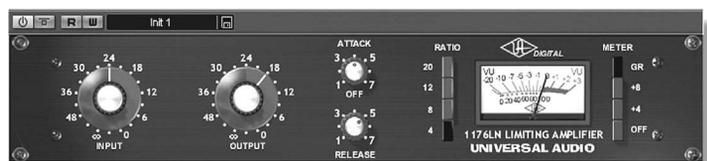
signal during the recording and/or mastering phase should only be used to remove occasional high-level peaks, as excessive use would trigger the process on successive peaks and would be noticeable. If the program contains too many peaks, it's probably a good idea to reduce the level to a point where only occasional extreme peaks can be detected.
