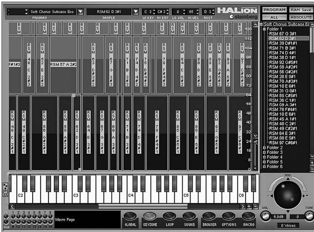
**Figure 4.11.** HALion 3 software sampling plug-in. (Courtesy of Steinberg Media Technologies GmbH, A Division of Yamaha Corporation; [www.steinberg.net](http://www.steinberg.net).)
