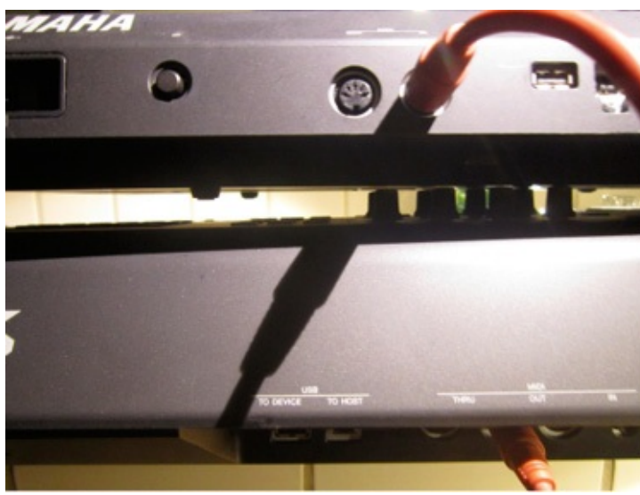
FIGURE 7.3. The most basic MIDI connection: A cable from a controlling device’s MIDI Out ( bottom ) connects to a receiving device’s MIDI In ( top ).
