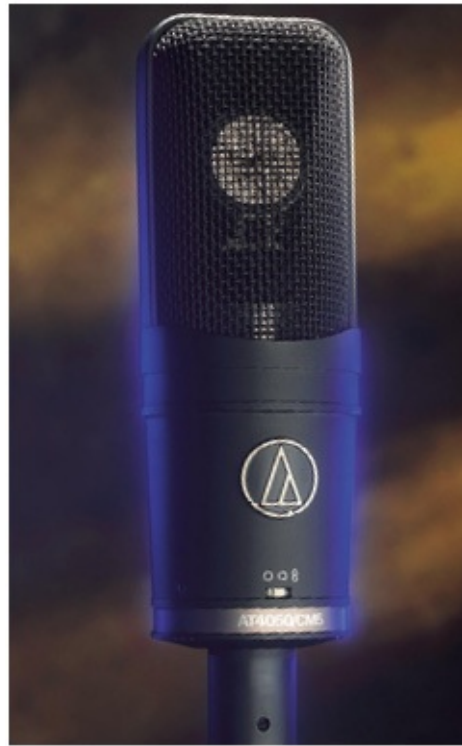
FIGURE 3.17. An Audio-Technica 4050, a condenser mic that can switch among cardioid, omni, or figure eight polar patterns. Photo courtesy of Audio-Technica.
