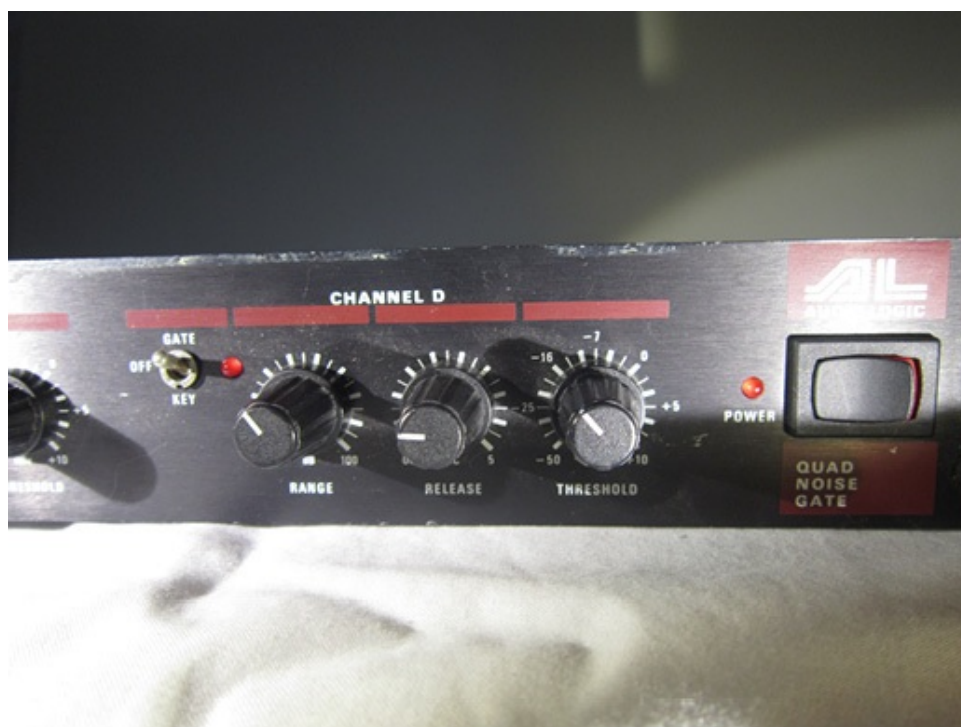
FIGURE 10.2. Front panel of a typical noise gate, showing range, release, and threshold controls.
