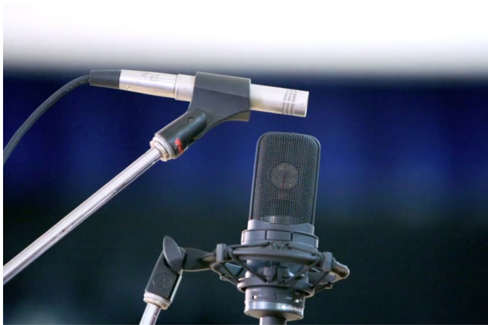
FIGURE 21.1. A Mid-Side microphone setup, with a figure eight mic at a right angle above the cardioid mic.
