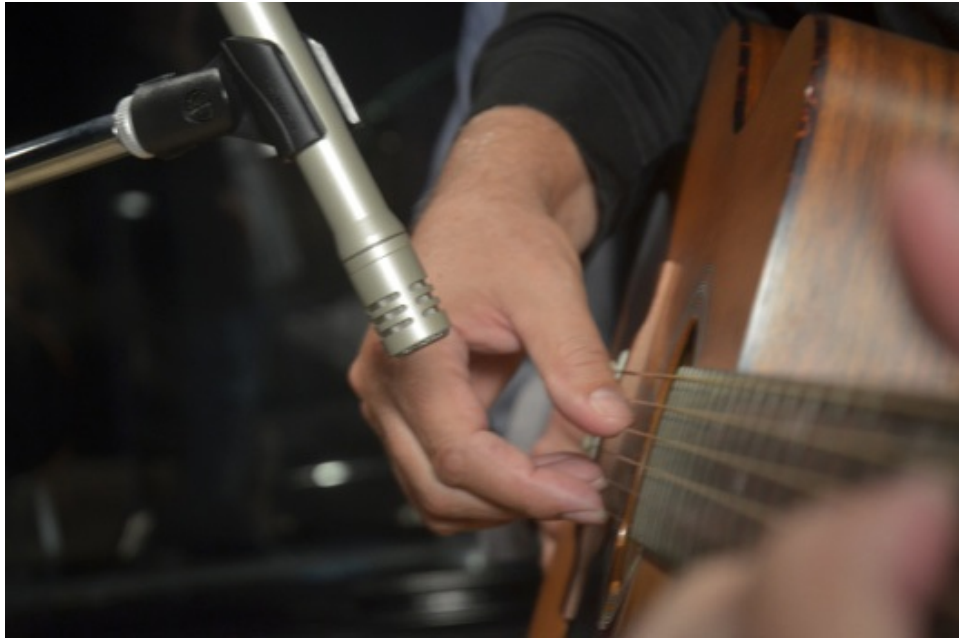
FIGURE 20.1. A guitar mic pointed downward, away from the vocal, to maximize the instrument's input. Photo by Charlie Steves.
