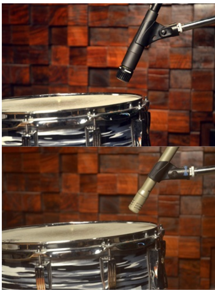
FIGURE 16.3. At the top is a classic snare mic—a dynamic—the Shure SM57. On the bottom is a small capsule condenser mic—generally the preferred choice of Alan. Photos by Charlie Steves.
