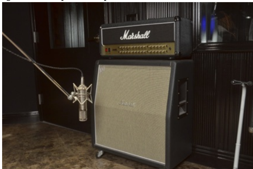
FIGURE 19.7. A condenser mic positioned a short distance from a Marshall cab.
