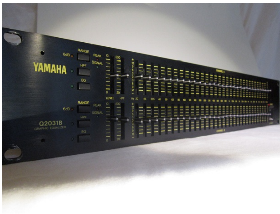
FIGURE 8.2. A stereo graphic equalizer with a “flat” frequency response, with all sliders/frequencies at 0 dB.
