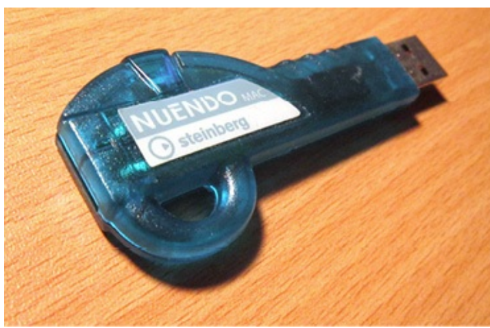
FIGURE 5.2. An iLok USB dongle for Nuendo, a high-end DAW used mainly in post-production.
